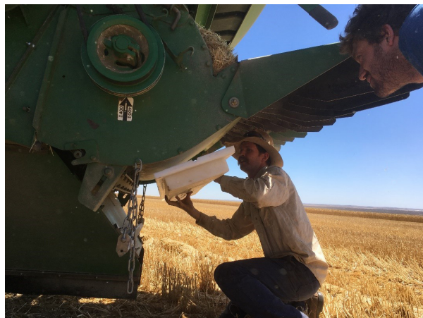
Attaching the ScherGrain harvest loss tray to measure rotor loss by collecting residue spread by the chopper
